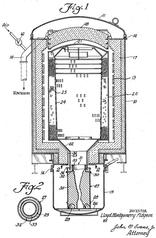
APPARATUS FOR PRODUCING MAGNESIUM
