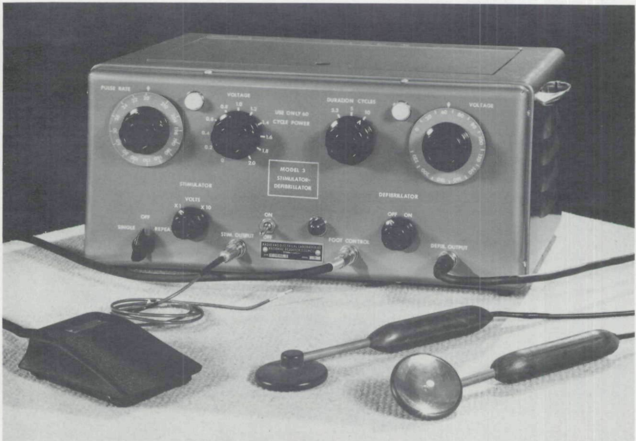
Figure 9. The combined stimulator-defibrillator designed by Jack Hopps and produced by the National Research Council in Ottawa. A foot pedal to trip the single 200 volt defibrillating shock and special electrodes that are held on either side of the heart to conduct the electric current through the organ are noted. National Research Council, 1950.
