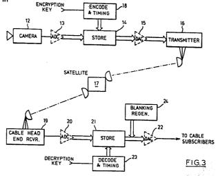
"METHOD FOR ENCRYPTING A LINE-SCANNED TELEVISION SIGNAL AND ENCRYPTING AND DECRYPTING APPARATUS"
