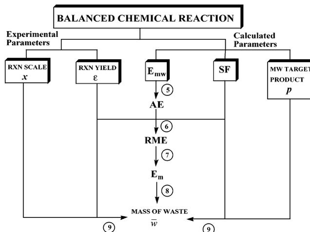
**Figure 1.** Flowchart showing interconnections between kernel and peripheral reaction metrics for a single general chemical reaction under conditions where the solvent and any catalysts are recycled or reclaimed. Circled numbers refer to corresponding equation numbers in text.
