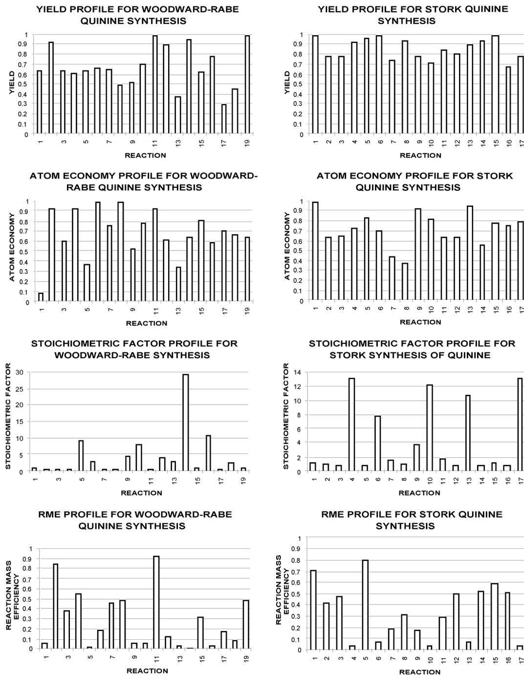
**Figure 3.** Yield, atom economy, stoichiometric factor, and reaction mass efficiency profiles or reaction maps for Woodward–Rabe and Stork syntheses of quinine. Reaction mass efficiencies are determined using eq 13.
